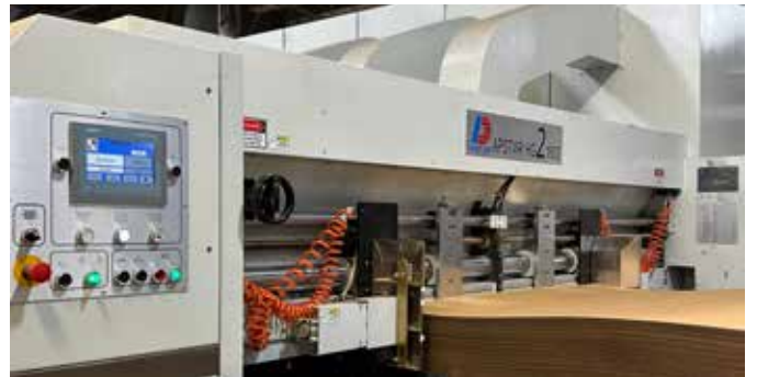
The Apstar's extended and print feed sections. Inline sheet cleaning and chamber ink metering with twin ink pumps has allowed Vineland Packaging to grow its marketing opportunities.
