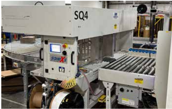
The SQ4 can strap and bundle up to 24 units per minute.
