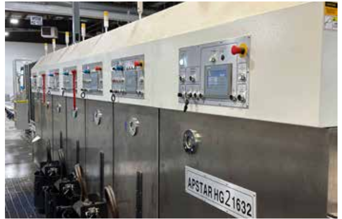
The Apstar's extended and print feed sections. Inline sheet cleaning and chamber ink metering with twin ink pumps has allowed Vineland Packaging to grow its marketing opportunities.
