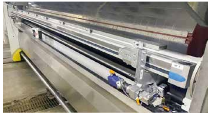
Vineland Packaging added JB ColorDry dryer units (above) and JB KleenPlate 3.0 (below) to its Apstar Rotary Die Cutter.
