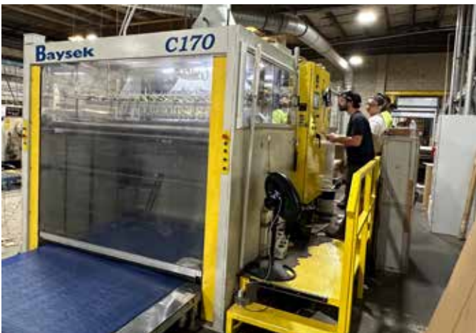
A Baysek C170 has been a die cutting workhorse that has been on Vineland Packaging's production floor for years.
