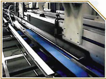
Creasing roller knife at final folding section for improved score lines and precise final folding
